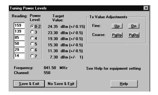
**Note:** The default cable loss 0.7 dB is taken into account in the values. If some other cables are used please, input the new value by using frequency planning.
