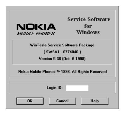
If WinTesla cannot find the file, op\_id.val, which contains the Login IDs, then the **OK** button will be 'grayed'. Otherwise, press the **CANCEL** button and only the Fault Logging feature of WinTesla will be deactivated.
