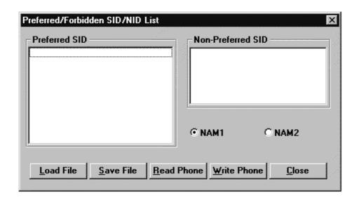
This option allows you to edit the SID list. Highlight entry using the <TAB> key and press <Enter> to edit.
