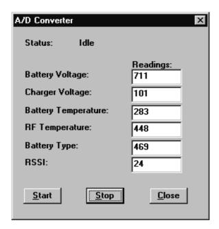
This option allows the phone's ADC readings to be displayed. The readings are updated every few seconds. There may be some delay before the mouse or keyboard responds while running this test.
