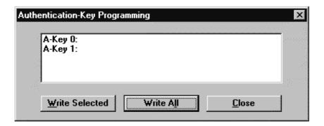
This option allows you to program the Authentication key (A–Key) of the phone. The A–key can *never* be read from the phone, only programmed to the phone over writing the previous value.
