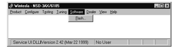
This command is used for flashing new software into the phone. While flashing the phone, user is shown the flashing progress towards completion.
